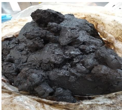
Figure 1 – Physical aspect of the solid material that was clogging the surface line in the offshore X field.
