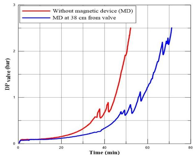
Figure 3 – Increase of differential pressure between the valve inlet and outlet due to scale formation with and without magnetic device.
