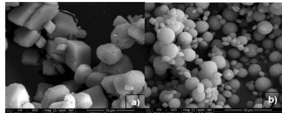
Figure 1 - a) Calcium Carbonate without the presence of magnetic field: Calcite; b) with the presence of magnetic field: CaCO<sub>3</sub> Vaterite)-Souza Junior, JR.
