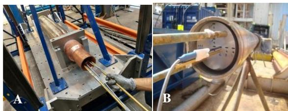
Figure 5 – Measurement of magnetic field just after the shock test (a), the metallic support (b) highlighting the seven positions that can be measured, and the three gaussimeters.
