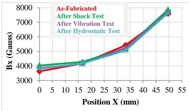
Figure 6 - Magnetic Field Density variation as-fabricated and after Shock, Vibration and Hydrostatic tests for the 5.5" Magnetic Device.
