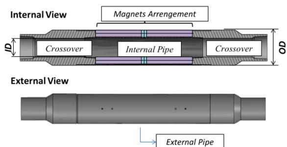
Figure 4 – 5 ½" Magnetic Accessory as-fabricated
