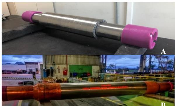
Figure 5 – Magnetic Arrangement (a) and 5 ½" Accessory as manufactured (b).
