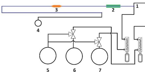
Figure 2 – Experimental loop for investigation of calcium carbonate scaling in saline oil emulsions under applied magnetic fields. Labels: (1)- mixture point, (2)- magnetic device, (3)- valve, (4)- waste tank, (5)- water tank, (6)- brine tank, (7)- emulsion tank.
