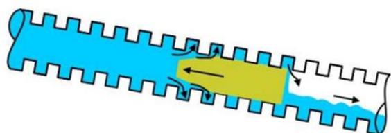
Figure 9: Water fallback in flexible line.
