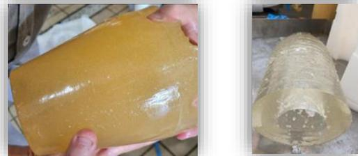
Figure 6: Pre-qualified gas-liquid spacers at laboratory scale: TINA on the left and CRIS on the right.
