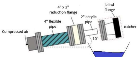
Figure 8: Schematic of the 4"x2" reduction apparatus.
