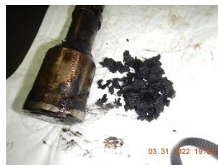
Figure 5. Solid sample retained from W1 during impression block tool run.
