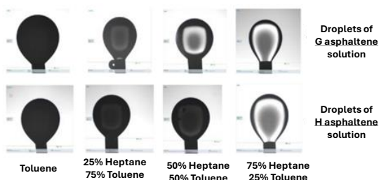
Figure 3. Images of drops of G and H asphaltene solutions in heptol containing different proportions of heptane and toluene – Surrounding phase: NaCl 1M, T = 60°C and P atm
