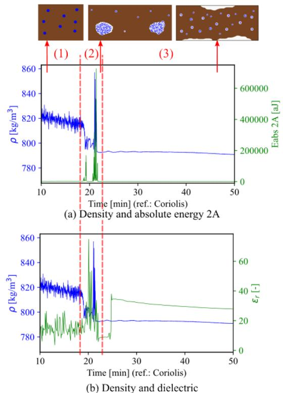
Figure 2. Density synchronized, in relation to the Coriolis, with (a) the absolute energy from probe 2A and (b) with the dielectric
