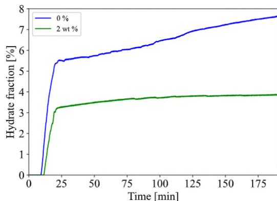
Figure 4. Hydrate fraction as function of the time and wax fraction (0 and 2%) at 400 L/h
