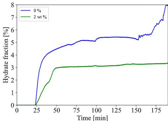
Figure 3. Hydrate fraction as function of the time and wax fraction (0 and 2%) at 200 L/h
