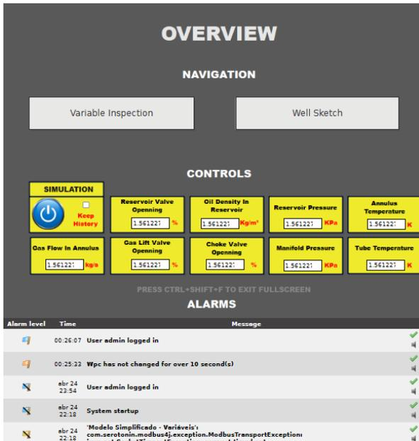
Figure 1. Screen control and navigation area.
