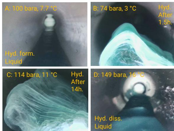
Figure 3. Test with CO<sub>2</sub> + N<sub>2</sub> + C1 mixture and 10% water for gas hydrate formation under static conditions. The line colors correspond to the different segments of the experiment.
