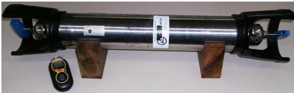
Figure 4: The model fluid was combined in a floating piston bottle at 9000 PSIG.
