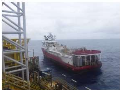
Figure 4. WSSV approaching SPU to perform the acetic acid 10% treatment. The acidizing operation was performed to optimize the removal of inorganic Scale. The acidizing and well return sequence to production is shown in Figure 5.
