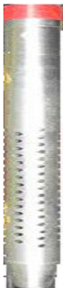
Figure 1. A Silver-Hawg Wax Inhibiting Tool (Sulaimon, et al. 2010:27)
