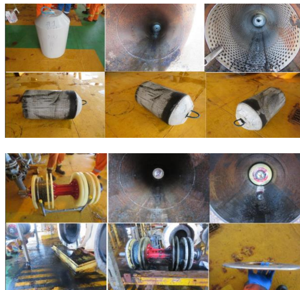
Figure 7. 2021 Mid-life pigging: Before and after pictures of the 4% Bypass Foam Pig (Top) and 2% Bypass Brush Pig (Bottom)
