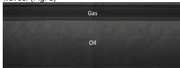
Figure 3. Smooth stratified flow pattern observed in the acrylic window
