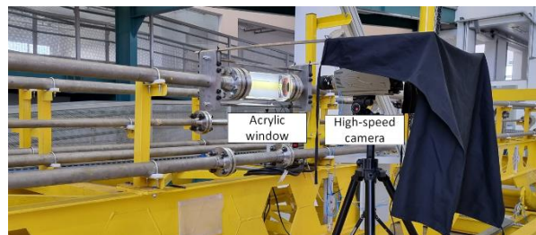
Figure 2. Two-phase dense-gas/liquid flow being recorded by the high-speed camera
