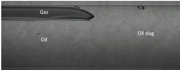
Figure 5. Intermittent flow pattern observed in the acrylic window
